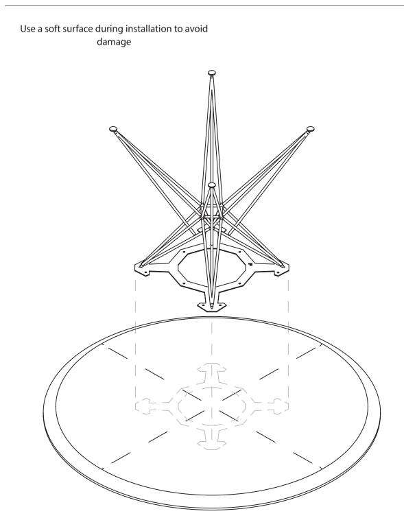
Place the tabletop upside down on a soft surface (e.g. a rug) to prevent scratches.
