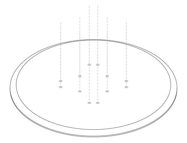
Mark the holes on the table top and remove the hairpin frame from the table top.
