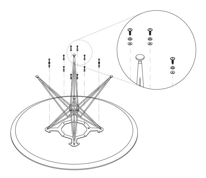
Place the frame with the mounting plate on the table top again and align it with the holes.
