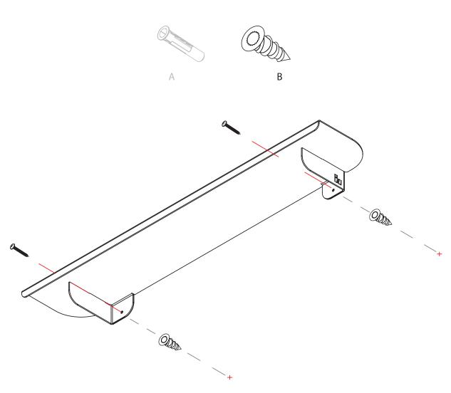
Screw the plug into the wall with a screwdriver. NOTE: Use a bit that has the correct size.
