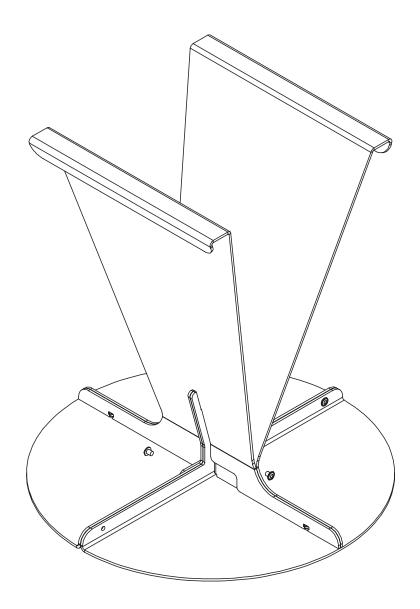
6. Tighten the inner allen bolts in the 2 holes using the allen key as shown above.
