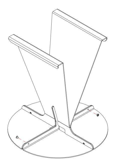
3. Tighten the outer allen bolts in the 2 holes using the allen key as shown above.
