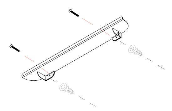
Screw the plug into the wall with a screwdriver. NOTE: Use a bit that has the correct size.
