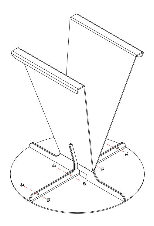
3. Push the screw with thread through the holes in the table top. Push on the other screw and tighten them (shown in red).
