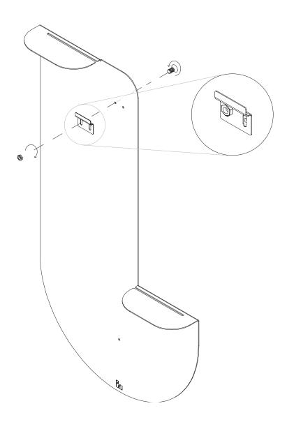
1. Mount the mounting plate to the steel base. Use the countersunk screw with M4 nut. Insert the bolt from the rear into the countersunk hole and attach the mounting plate by tightening the M4 nut.
