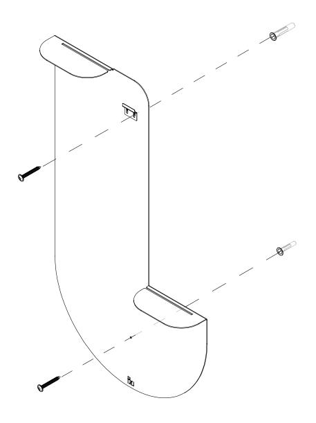
6. Attach the steel base to the wall with the supplied screws.
